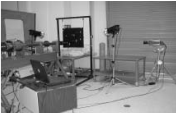
(a) A gas gun chamber is used to shoot a steel projectile to the composite plate
